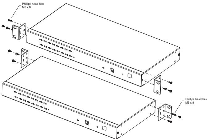
3. Slide the unit into the front or rear of the rack and secure it to the rack.
